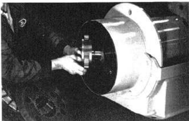
Remove sun gear shaft from final drive end (see final drive disassembly instructions). Remove primary planet assembly.
